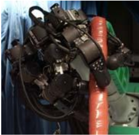
Figure (5) illustrates the painting robot holding a brush to draw with
